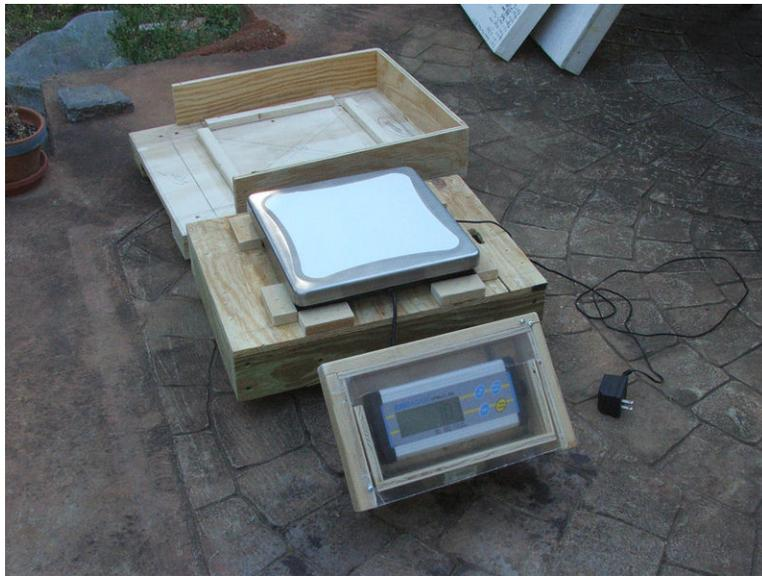
The scale on the platform with the top upside down. I built it so the scale was directly below the center of the hive reducing the chance of tipping over. The scale is connected to a computer using USB cables.
